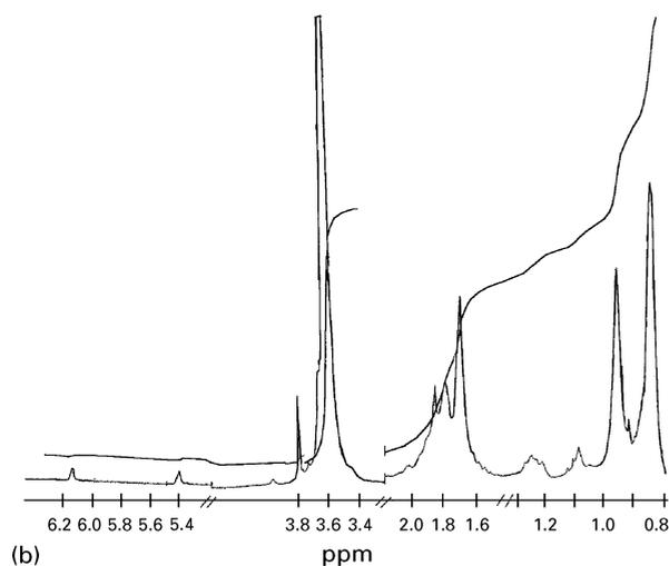
Figure 2 Proton NMR spectra of two formulations of bone cement prepared with (a) 0.75% and (b) 2% BPO concentration in the solid phase.
