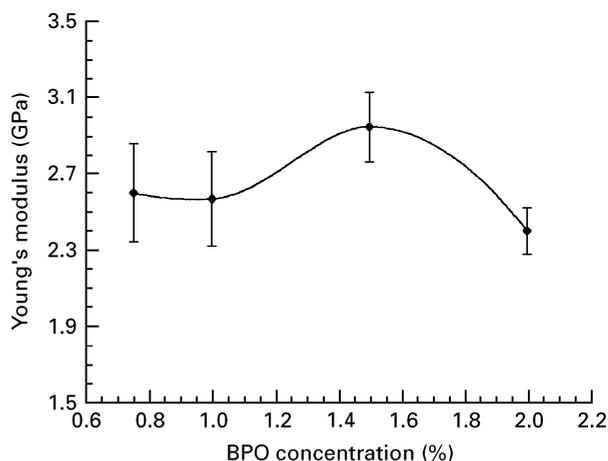
Figure 4 Young's Modulus (YM) as a function of the BPO concentration for an acrylic bone cement based on PMMA beads.
