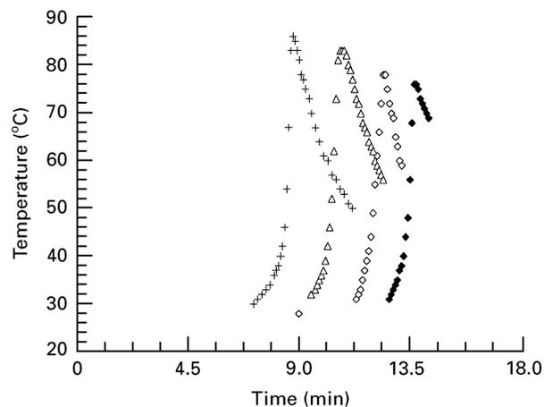
Figure 1 Polymerization exotherms of bone cement formulations prepared with 0.82% wt/wt of DMPTA and different concentrations of BPO:  $\blacklozenge$  0.75%,  $\diamond$  1%,  $\triangle$  1.5%,  $+$  2%.
