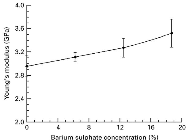
Figure 8 Young's modulus (YM) as a function of the barium sulphate concentration for an acrylic bone cement based on PMMA beads.
