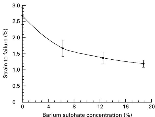
Figure 9 Strain to failure versus barium sulphate concentration for an acrylic bone cement based on PMMA beads.
