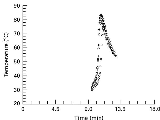
Figure 6 Polymerization exotherms of bone cements prepared with 1.5% wt/wt and 0.82% wt/wt of BPO and DMPTA, respectively, and different amounts of barium sulphate:  $\blacklozenge$  0%;  $\diamond$  6.25%; + 12.5%;  $\triangle$  18.75%.
