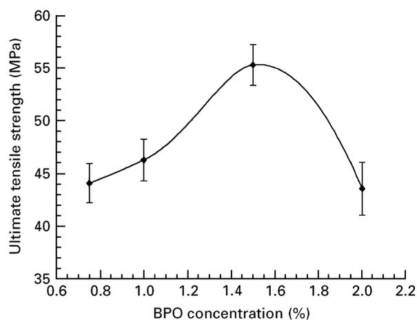
Figure 3 Ultimate tensile strength (UTS) versus BPO concentration for an acrylic bone cement based on PMMA beads.
