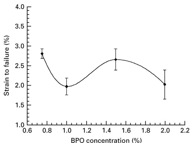
Figure 5 Strain to failure versus BPO concentration for an acrylic bone cement based on PMMA beads.
