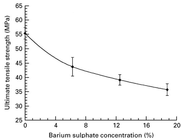
Figure 7 Ultimate tensile strength (UTS) versus barium sulphate concentration for an acrylic bone cement based on PMMA beads.
